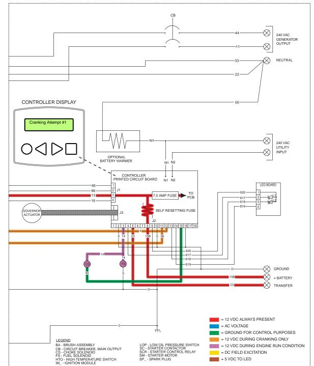
Figure 3. Circuit Condition - Engine Cranking
